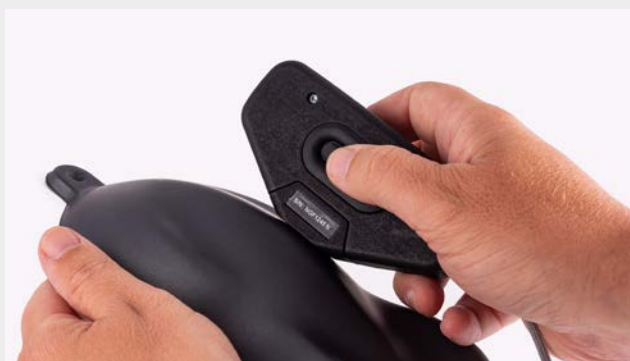
Measures curvature in both directions
